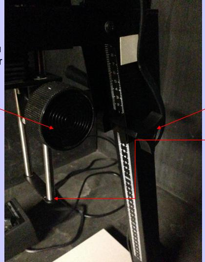
The triangular knob allows you to loosen the head of the enlarger to move it up and down to make the image larger or smaller, with the help of the handle, which you must hold until you retighten the triangular knob.
