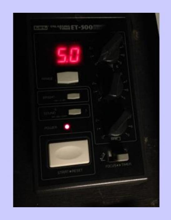
6. Cover your test strip with the black card exposing about a half inch to an inch piece. Expose your paper to the light with the timer for 5 seconds.
