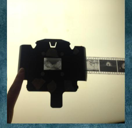
4. Put negative carrier with negative in it into enlarger with light off.
